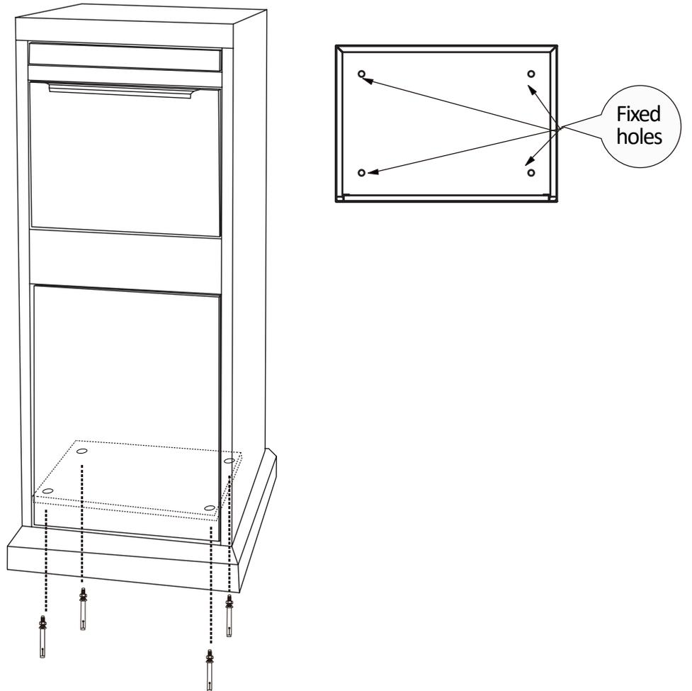
2. Please refer to the holes distance to drill the holes(depth 85mm, diameter 12mm) on the ground accordingly.
